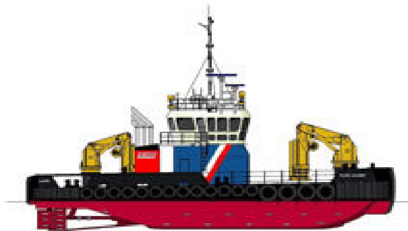
Forth Joustier. Length 26m. Beam 11.5m. Draft 2.35m Type: Multicat. Displacement 515 tonnes.
